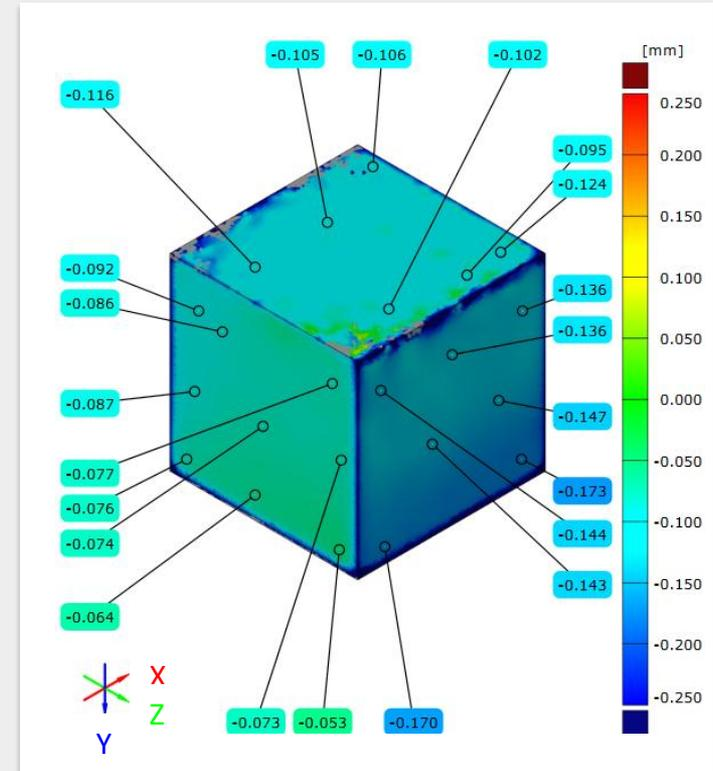
Test cube with uniform tooling factor 1,2
