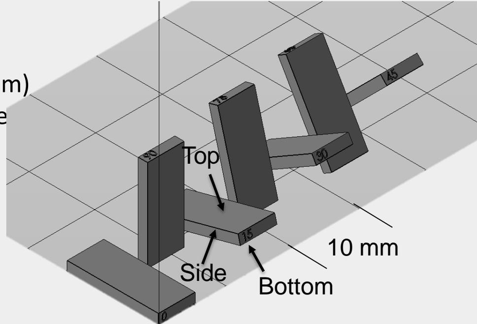
Surface roughness test parts
